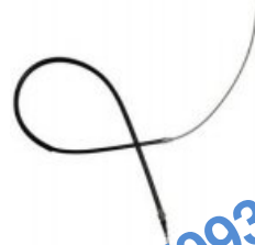
KP-VW-02207 BRAKE CABLE 357609721A Length [mm]:1749 Length 1 [mm]:1178 PASSAT
