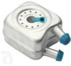
KP-VW-07001 OIL COOLER 000 117 021B 060 118 021 B Length [mm]:90 Width [mm]:90 Weight [kg]:0,66
