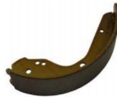
KP-VW-01063 BRAKE SHOE GS8149 251698531LV Diameter [mm]:252 Width [mm]:56 TRANSPORTER III BUS
