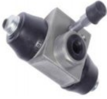
KP-VW-02032 BRAKE WHEEL CYLINDER 1H0 611 053 861 611 053 Diameter [mm]:19 POLO GOLF CADDY
