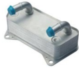
KP-VW-07016 OIL COOLER 02E 409 061B 02E 409 061B Length [mm]:190 Width [mm]:96 Core Dimensions:190x96x75 Weight [g]:400 Depth [mm]:75 NEW BEETLE GOLF V JETTA III
