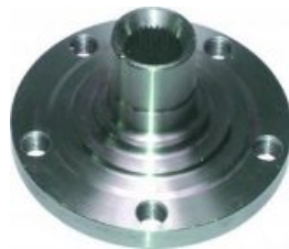
KP-VW-03018 WHEEL HUB 357501117 Inner diameter [mm]:109 Outer diameter 1 [mm]:29 Outer diameter 2 [mm]:17,4 Height [mm]:80 JDI80 JETTA I PASSAT GOLF
