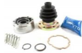
KP-VW-04324 CV JOINT ZBA407331 INNER AXLE JOINT GOLF I GOLF II GOLF III
