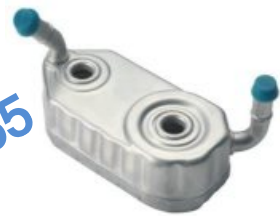
KP-VW-07008 OIL COOLER 030 409 061 096 409 061E 006 409 061C Length [mm]:189 Width [mm]:89 Core
