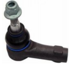
KP-VW-04052 TIE ROD END 7L0 422 817 B L=89 mm T1=M14X 1.5 T2=M16X 1.5 TOUAREG
