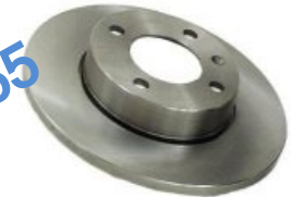
KP-VW-01176 BRAKE DISC 811615301 823615301 JETTA POLO GOLF PASSAT Diameter [mm]:239 Thickness [mm]:9,9 Minimum thickness [mm]:8 Height [mm]:38,5
