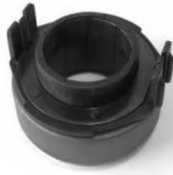
KP-VW-02070 RELEASE BEARING 969002514 002141165L Outer diameter [mm]:39,19 Inner diameter [mm]:25,43 CADDY
