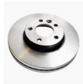
KP-VW-01172 BRAKE DISC 7H0615301D TOUAREG TRANSPORTER Diameter [mm]:308 Thickness [mm]:29,9 Minimum thickness [mm]:25,5 Height [mm]:55,5
