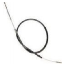
KP-VW-02215 BRAKE CABLE 191609721E Length [mm]:1527 Length 1 [mm]:1085 GOLF JETTA
