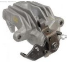
KP-VW-01097 BRAKE CALIPER 1J0615423D 1J0615423F GOLF IV NEW BEETLE
