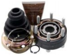
KP-VW-04321 CV JOINT 701498103 Joint diameter (mm):108 Length [mm]:31,8 TRANSPORTER IV
