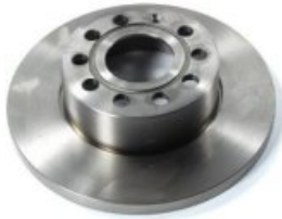
KP-VW-01197 BRAKE DISC 1K0615601L 1K0615601AC TOURAN GOLF JETTA CADDY Diameter [mm]:256 Thickness [mm]:12 Minimum thickness [mm]:10 Height [mm]:48,5
