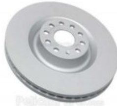
KP-VW-01202 BRAKE DISC 1K0615301M GOLF PASSAT Diameter [mm]:345 Thickness [mm]:30 Minimum thickness [mm]:27 Height [mm]:49,9
