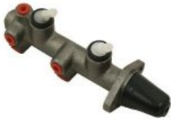
KP-VW-02009 BRAKE MASTER CYLINDER 113 611 015 113 611 016 149 611 015/2 Diameter [mm]:19,05 Thread Measurement 1:5xM10x1 KAEFER ILTIS
