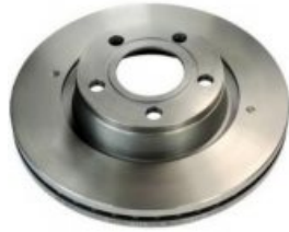
KP-VW-01170 BRAKE DISC 8E0615301B 8E0615301P PASSAT AUDI Diameter [mm]:280 Thickness [mm]:22 Minimum thickness [mm]:20 Height [mm]:46,23
