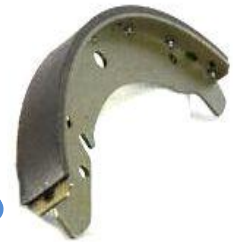
KP-VW-01064 BRAKE SHOE GS8028 131 698 537 CX Diameter [mm]:230 Width [mm]:30 KAEFER
