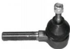
KP-VW-04069 Tie Rod End 113415821 / 113415821A Kaefer/Beetle Kaefer / Beetle Cabrio (Typ 1) Karmann Ghia Cabrio (Typ 1)
