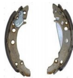
KP-VW-01056 BRAKE SHOE 867698525 171609527 191609525 Diameter [mm]:180 Width [mm]:30 PASSAT POLO II III JETTA AUDI
